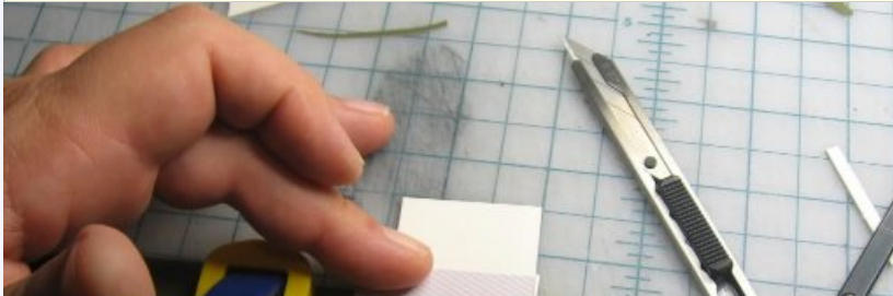
Turning the whole thing over, and I used the tool to cut out a former of constant thickness (it helps to clamp the work down to keep it from moving). Each successive cut leaves behind the same shape that the tool fits in. Repeatability is the goal:
